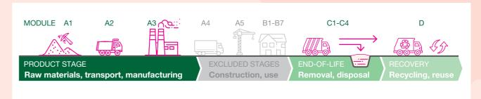
The production stage (Modules A1-A3) includes all aspects of Comfortech® insulation production from cradle to gate, utilising elementary and product flows. End-of-life stage (C1-C4) and benefits beyond the system boundary (module D) are included according to the mandatory requirements of EPD.
