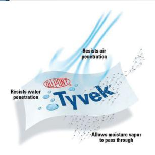
DuPont™ Tyvek® Supro is a self-supporting, fire retardant synthetic roof underlay, made by laminating a spun-bonded high-density polyethylene (HDPE) to a non-woven polypropylene sheet. This provides a strong weather resistant barrier with excellent water vapour permeability.
