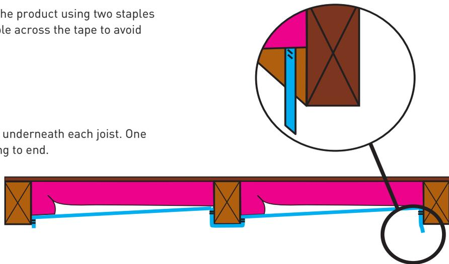
**When installing around electrical cables ensure that you have a clear view of the joist face. Avoid stapling close to electrical wires.**
