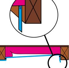
When installing around electrical cables ensure that you have a clear view of the joist face. Avoid stapling close to electrical wires.
